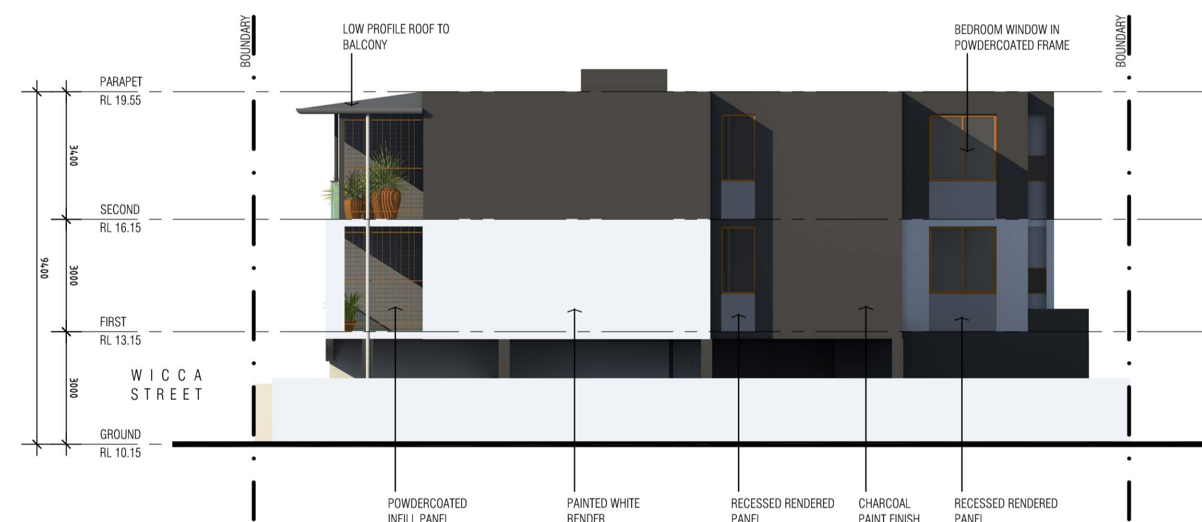
SOUTH WEST ELEVATION
